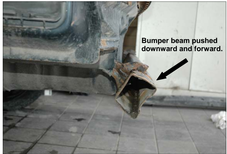
...Structural damage visible when cover removed
