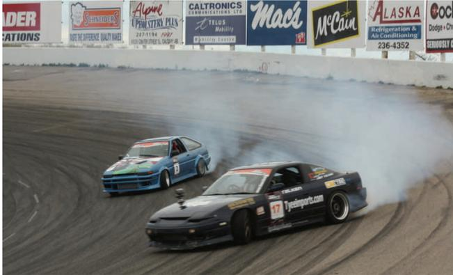
Tire marks left by drifting are different than most marks found in accident reconstruction because throttle is applied through the slide. In an accident it is usually the opposite, and brakes are applied. Drifting yaw marks are usually thick and black whereas normal yaw marks usually show lateral striated marks as the tires are spinning at a slower rate.
