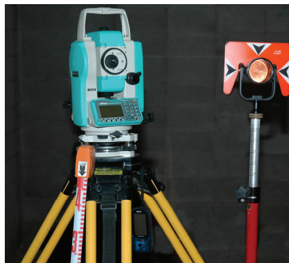
Survey Total Station
