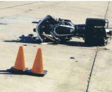
**Airborne Trajectory:** Frequently, the impact involves a vehicle turning left across the path of a motorcycle. If the rider becomes airborne, a speed can be calculated. The calculation requires the rider take-off angle and height (via inspection of the bike), and the distance the rider is
